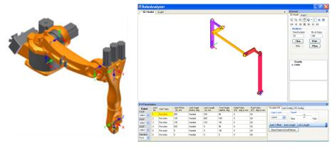
(a) Assembly in Autodesk Inventor Figure 5: KUKA KR5 robot
