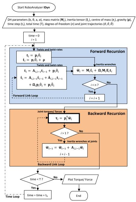
Figure 3: Flowchart of IDyn algorithm
