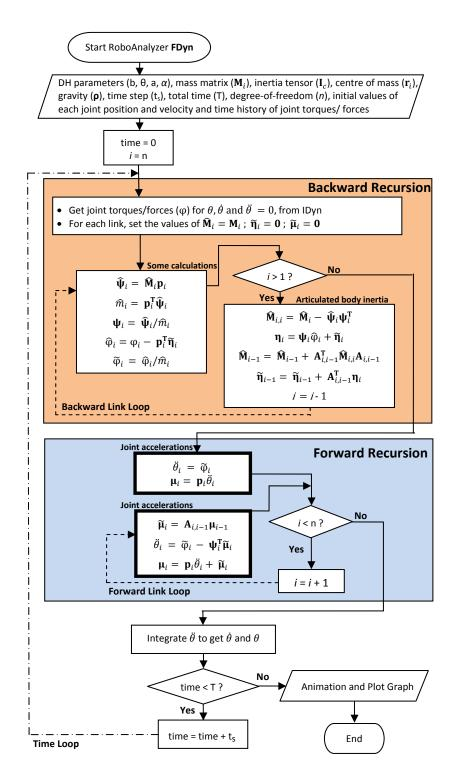
Figure 4: Flowchart of FDyn algorithm
