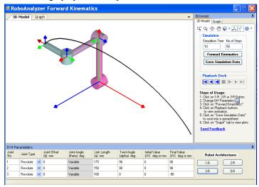
Figure 1: RoboAnalyzer animation of a 3 degree-of-freedom serial manipulator
